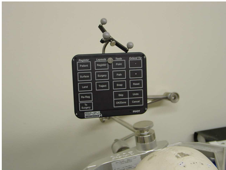
Figure 6: Virtual, tracked, keypad (courtesy N. Glossop, Traxtal technologies).
