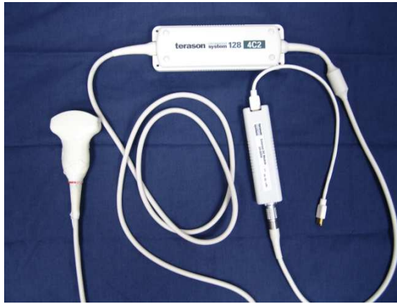
Figure 3: The Terason compact ultrasound system from Teratech Corporation (MA, USA). Image shows all hardware components. System connects via IEEE-1394 (Firewire) to a laptop.
