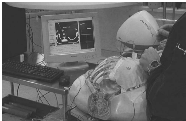
FIG. 5. A radiology resident is using the electromagnetic navigation system to guide the needle into the nodular target using the GUI. A typical puncture starts with path planning followed by needle puncture algorithm which displays a graphical representation of the needle on the GUI in real time.
