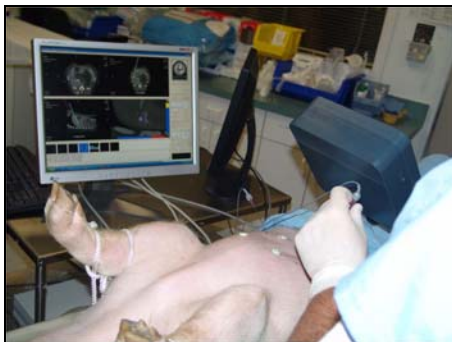
Figure 2: Swine study in CT (GUI at top left, swine at bottom left, electromagnetic tracker on right)
