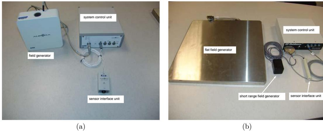
**Figure 3.** Electromagnetic tracking systems and their components, as used in this study, (a) Aurora and (b) 3D Guidance.
